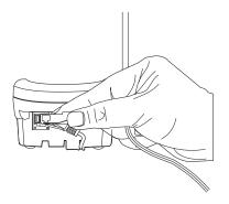
4. Place the telephone cord inside the molded channel on the bottom of the Base Unit.
